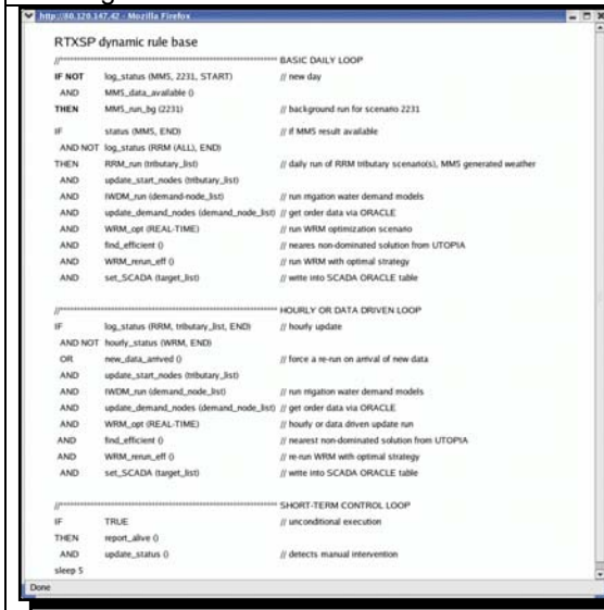
Figure 9: Rule-base for the real-time optimization and heuristics
